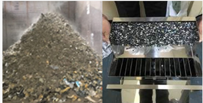
ASR (left) and the resin extracted from it (right).
